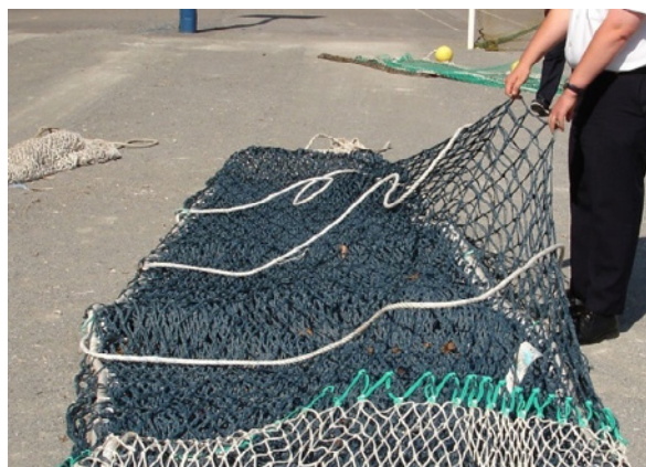
Figure 76 – Fourreau de renforcement
