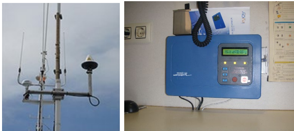
Figure 30 – Examples of a VMS antenna (left) and transceiver (right)
