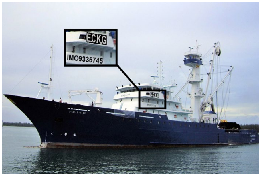
Figure 22 – Example of an IMO number on a fishing vessel
