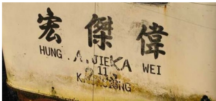
Figure 18 – Example of confused marks on the stern of a longliner
