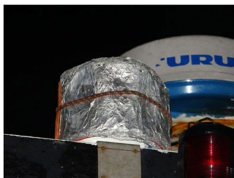
Figure 31 – Example of a masked VMS antenna
