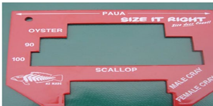
Figure 46 – Example of a vernier shellfish gauge
