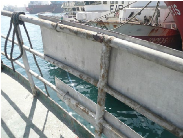
Figure 20 – Example of removable plaques for the registration number and vessel name
