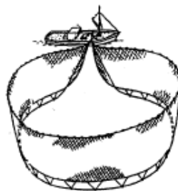
Figure 57 – Retrieval of a purse seine
