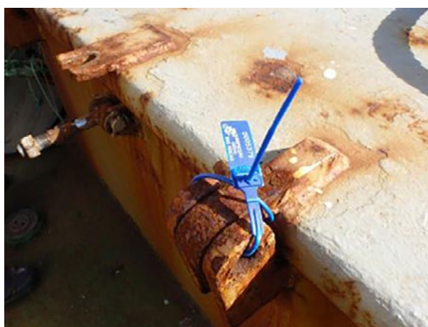
Figure 89 – Example of sealing of access to the hold
