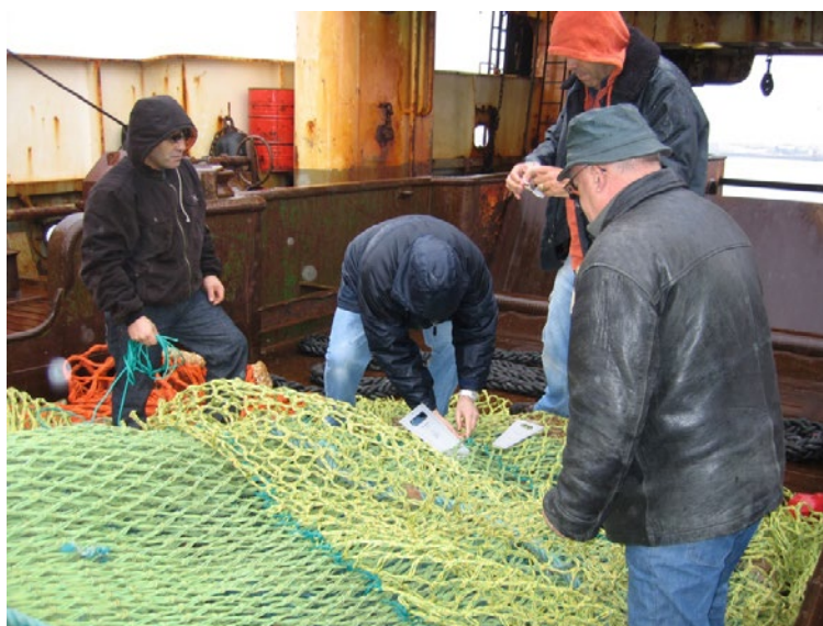
Figure 73 – Measuring mesh size of a trawl
